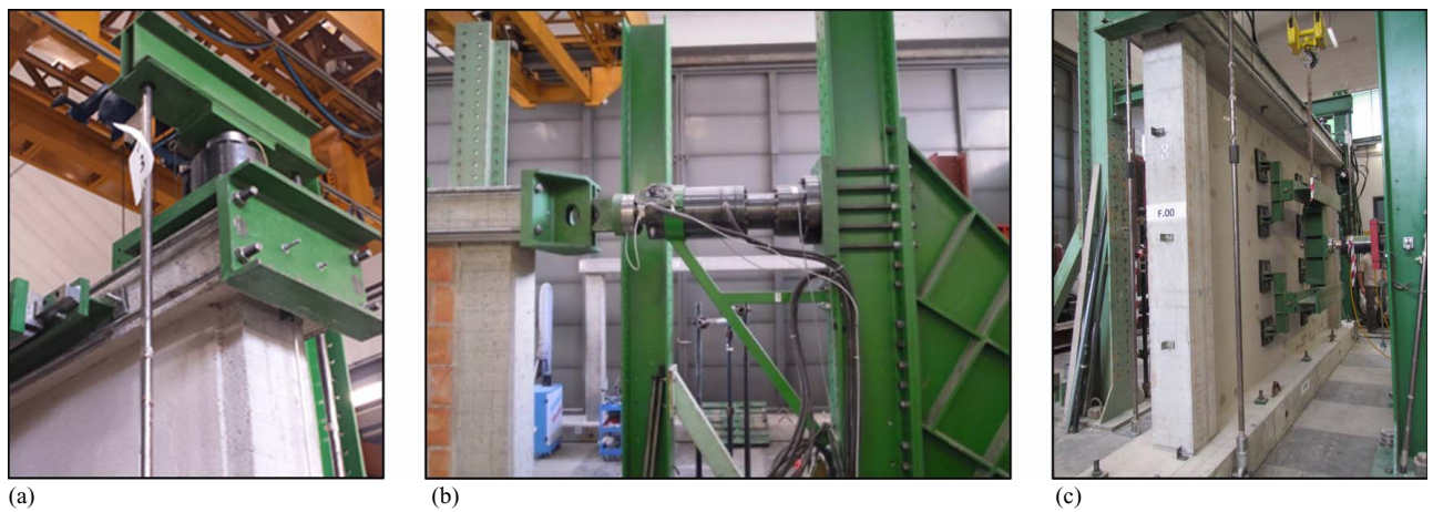
Fig. 9. Experimental setup: (a) actuators for vertical loading; (b) actuator for IP horizontal displacements; and (c) OOP thrusting system.
