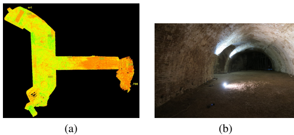
Figure 1. (a) Top view of Impossibile bastion, walls of Padova, Italy. Terrestrial laser scanner 3D reconstruction obtained with Leica ScanStation C10. (b) Inside view of the bastion.
