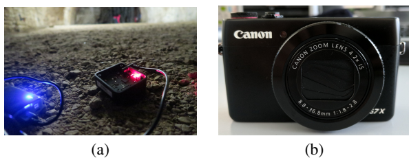
Figure 2. (a) UWB Pozyx device powered by a standard powerbank. (b) Canon G7X camera.
