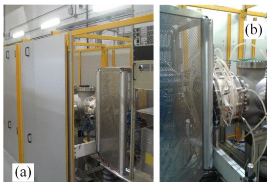
FIG. 2. (a) View of the NIO shielding box with main door open and main rf generator removed; (b) accelerator column and HVD view from the opposite side.
