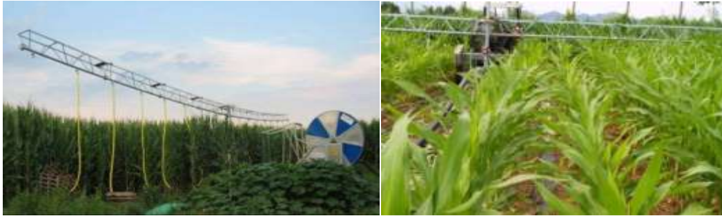
Fig.1 and 2: Traveller boom with and without drop tubes to apply water into the soil under the canopy
