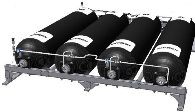
Fig. 6. Four tanks occupying a volume of 3.4 \text{ m} \times 2.2 \text{ m} \times 0.52 \text{ m} can store 1900 liters of hydrogen at 35 MPa (30.9 kg), sufficient to supply a fuel stack delivering 500 kWh of electrical power (courtesy of Nuvera®).
