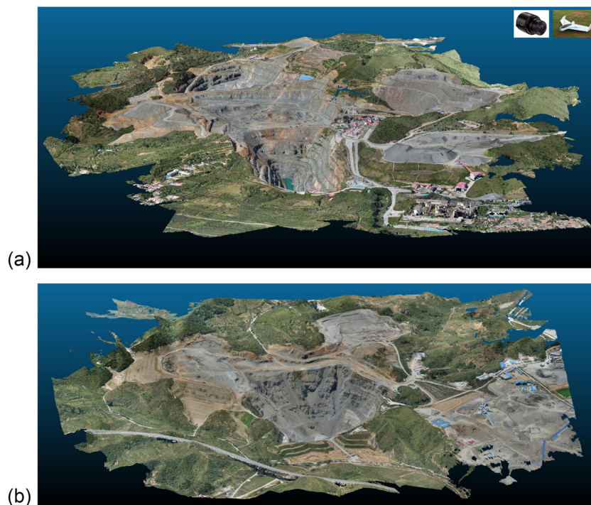
Fig. 3. 3D-view of the point cloud with coupled RGB colours for the surveyed mines I (a) and II (b). In addition, notice a detail regarding the UAV used for the survey over the iron mining area and the mounted Sony Cyber-shot DSC-QX100 camera for the photograph collection.
